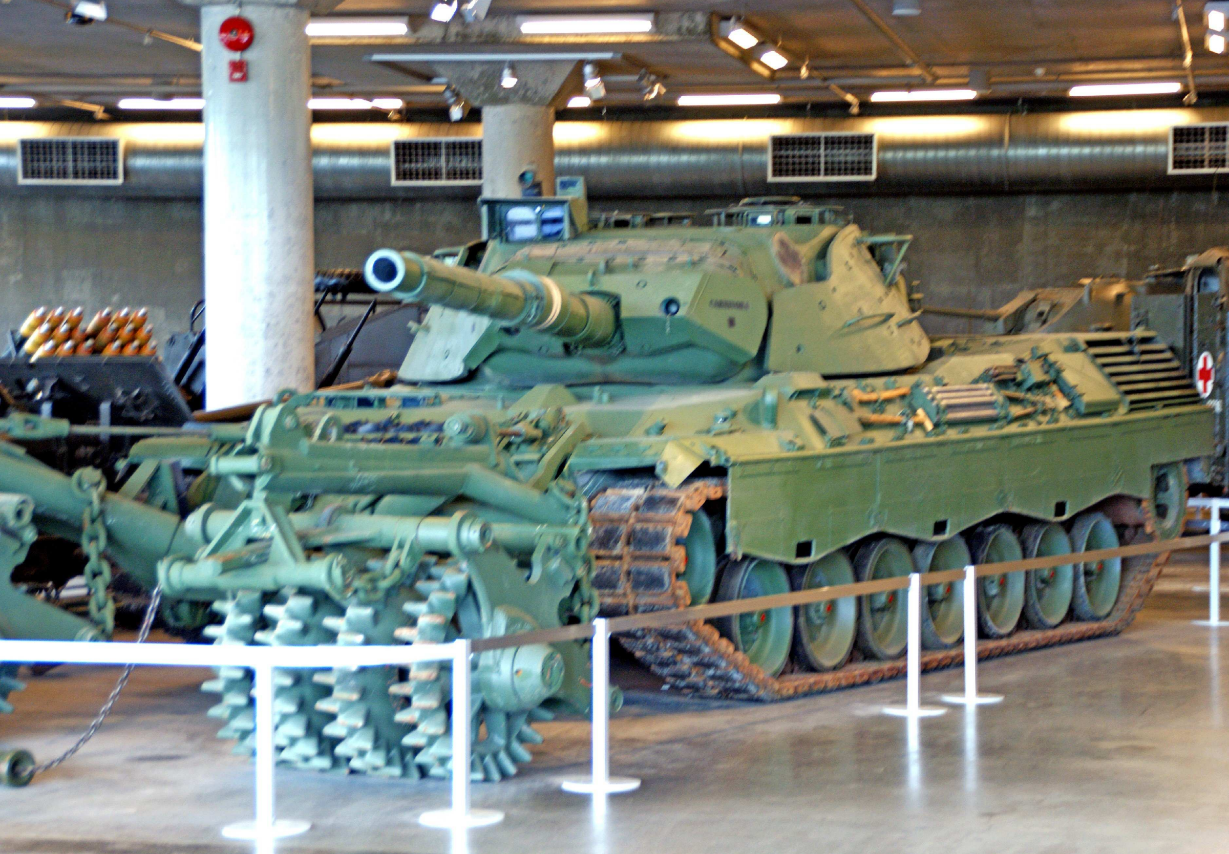
Canadian Army (German design) Leopard 1C2 tank with mine-clearing rollers used in the 2001-2014 Afghanistan war.
